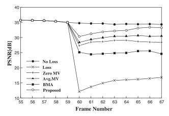
Figure 2: Error propagation comparison of Carphone concealed by conventional methods and proposed method.
